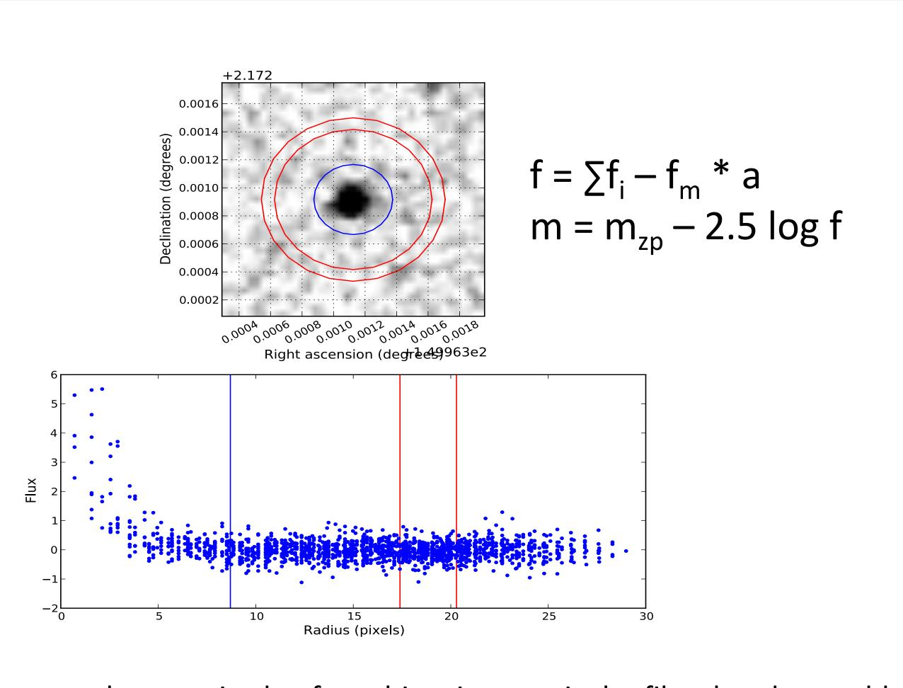
To compute the magnitude of an object in a particular filter band, we add up the flux of all of the flux in a circle around the object (blue circle), and subtract the median sky pixel (in the red annulus) multiplied by the area of the blue circle to get the total flux. Magnitude is a logarithmic scale of the total flux scaled to a zero point given in each image. This can then be compared with other bands and other telescopes.
