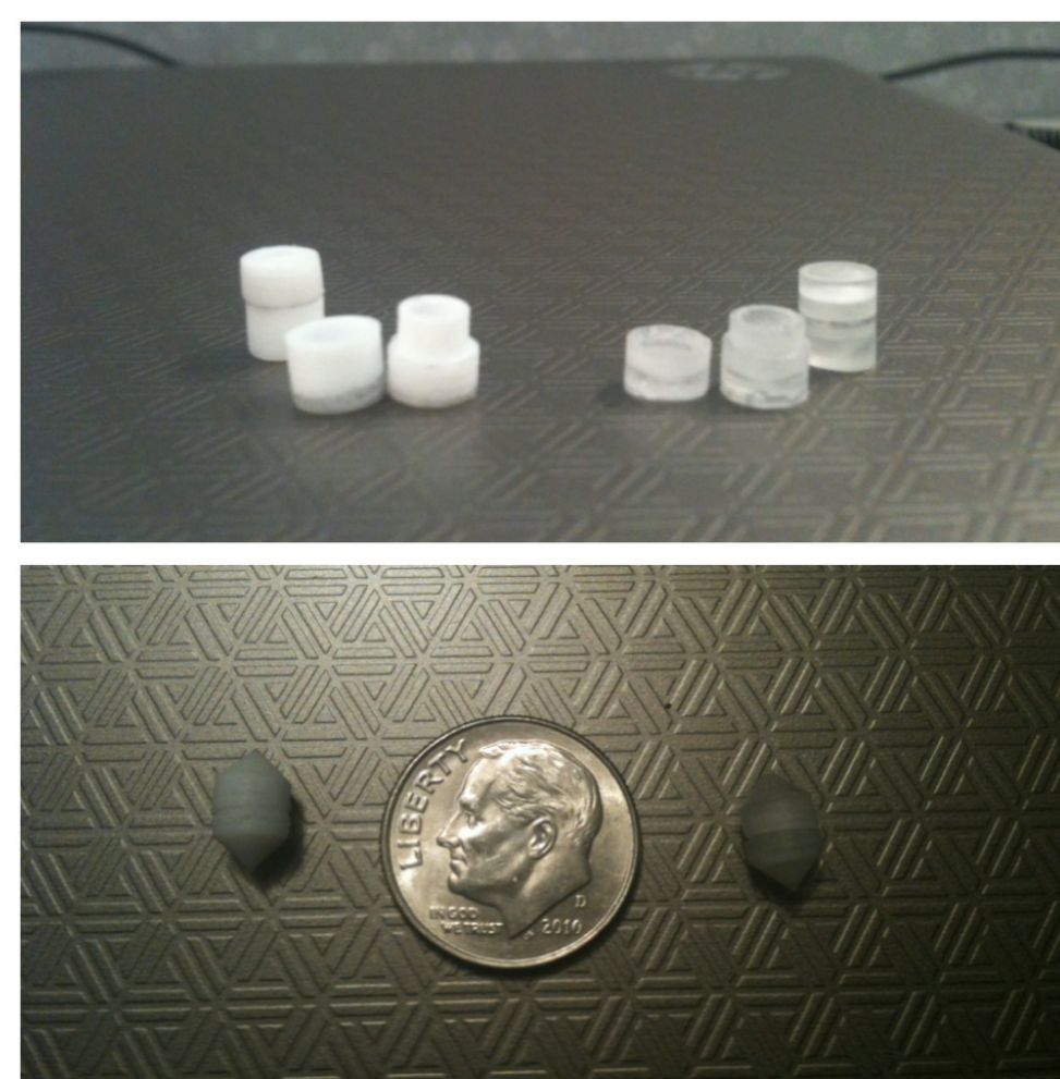
The original holders in Teflon and Rexolite (top), and the double cone holders (bottom)
